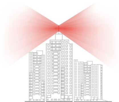
Figure 3.1 – Correct antenna installation position
